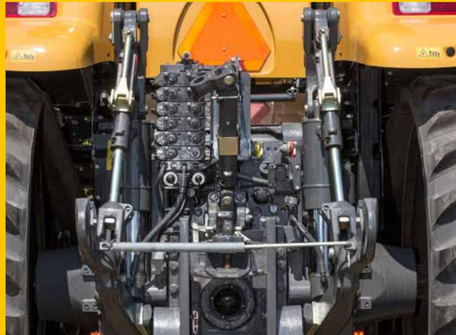
Three-point linkages are designed as an integral system to provide maximum lift capacity, lift height and control. The standard 3-pt. linkage on the MT700E also features a lift capacity in excess of 81.7 kN, with a maximum lift capacity of 130.9 kN. This provides the greatest lift capacity at the implement's centre of gravity, where it's needed most. For longer service life, inverted, seal down lift cylinder ensure clean and debris-free operation.
