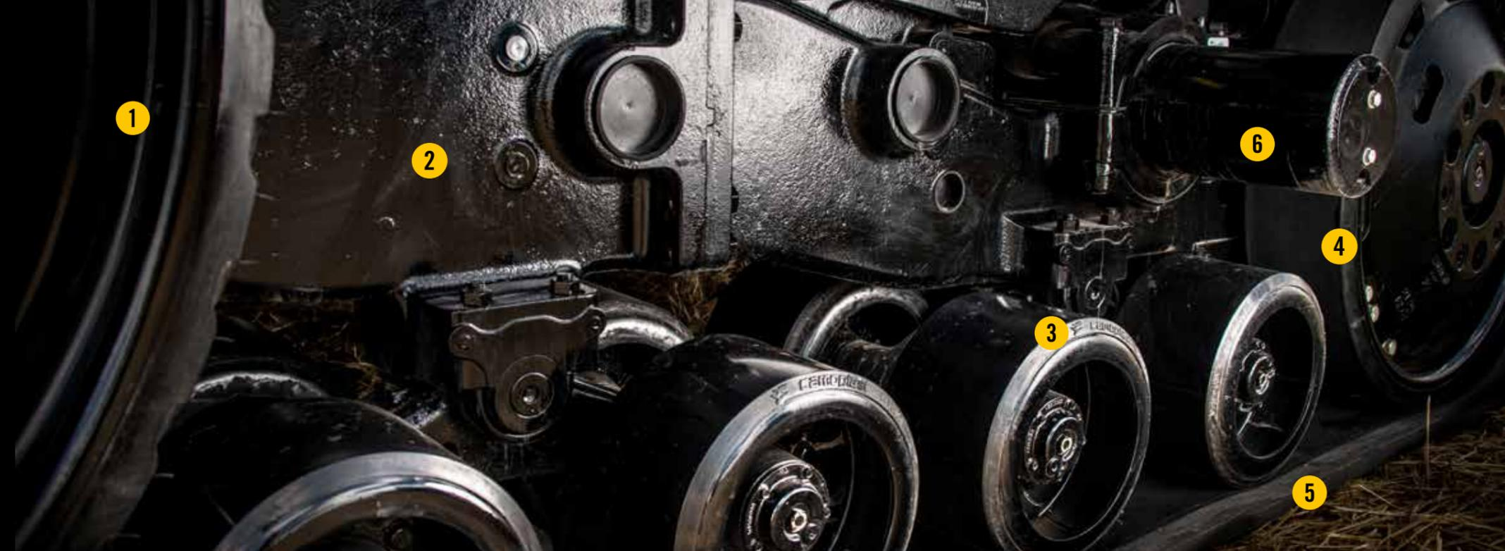
**1** Lower rolling resistance, plenty of driver to belt grip and easier walk over bumps are among the benefits of the large diameter driver, the largest in its class. The wide chevron grooves on the surface of the driver wheels optimize mud rejection and driver grip.
